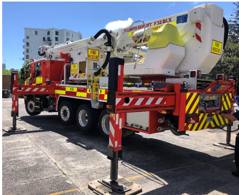
Figure 13 – Highlights the space requirements for jacking stabilisers
