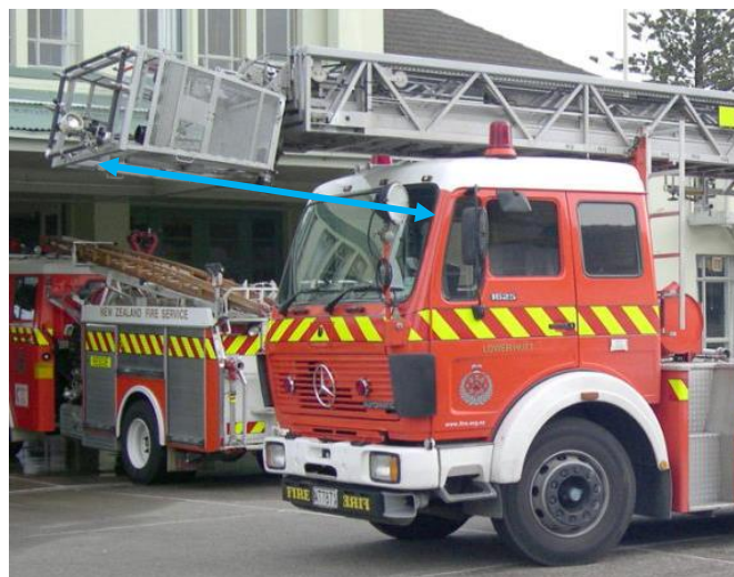
Figure 5 – Showing long front overhang
