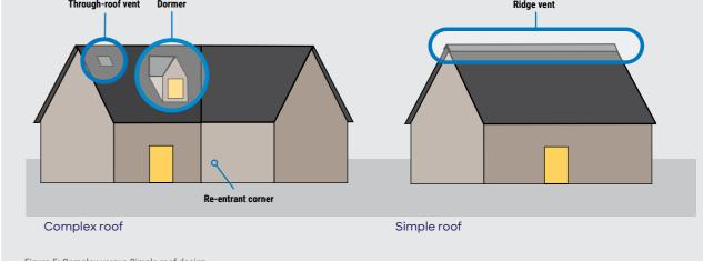
Figure 5: Complex versus Simple roof design
