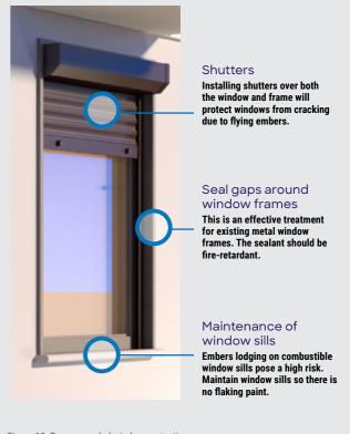
Figure 13: Recommended window protection
