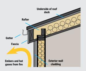
Figure 8: An eave with essentially no overhang versus an enclosed overhang with horizontal soffit
