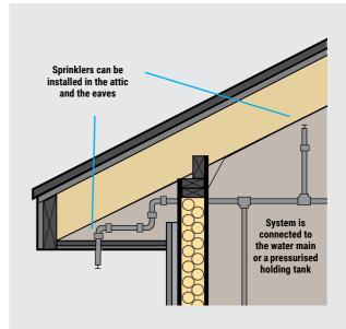
Figure 18: External and home sprinkler can be installed in conjunction with
