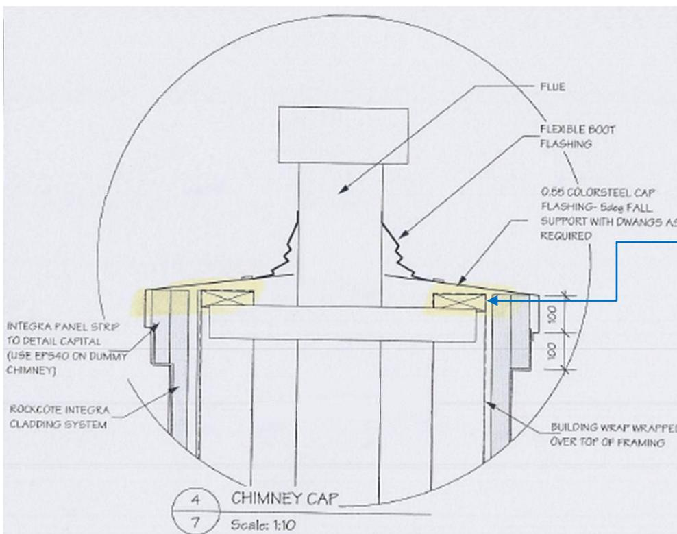
In one case the fire investigator was able to confirm the chimney chase had been built to the architectural requirements. Non-combustible material was not specified beneath the flashing.
