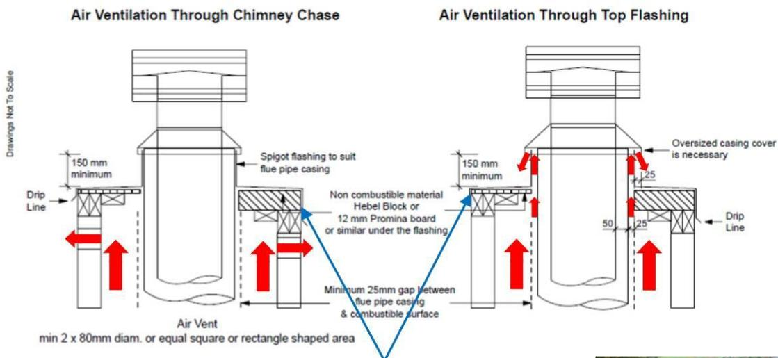
Above - A manufacturer's specification requiring non-combustible material immediately under the flashing.
