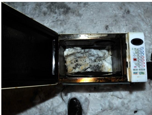
Results of an overheated wheat bag which was inadvertently heated in a microwave oven for 20 minutes
