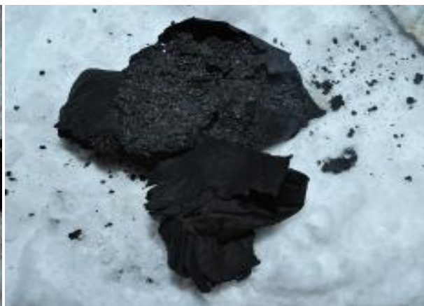
Results of an overheated wheat bag which was inadvertently heated in a microwave oven for 20 minutes
