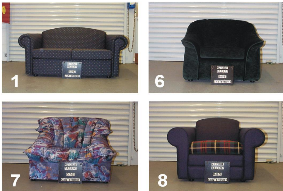
Figure 10 - Photographs showing the items of furniture burned in the flame height experiments. Item 1 is the two-seat version of the sample tested and is representative also of items 2 to 5, with only the fabric varying.
