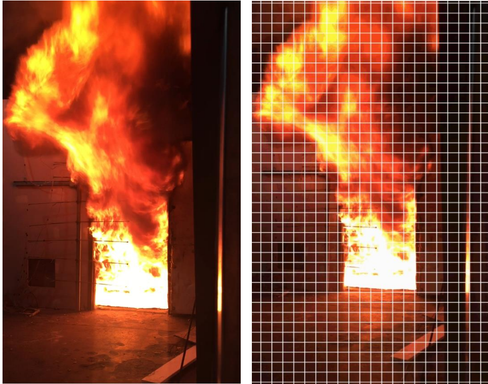
Figure 14 - Video image of the flame compared to the same image with the analysis mesh overlaid on the video image.
