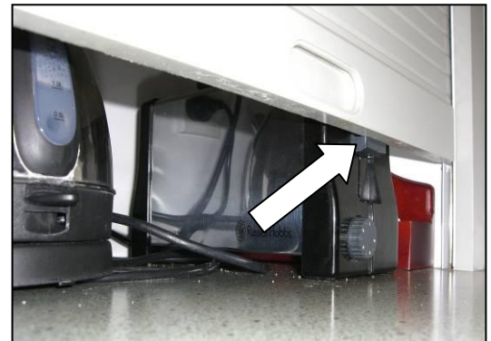
Right: A toaster with it's on/off lever trapped by the door of an kitchen appliance garage.
