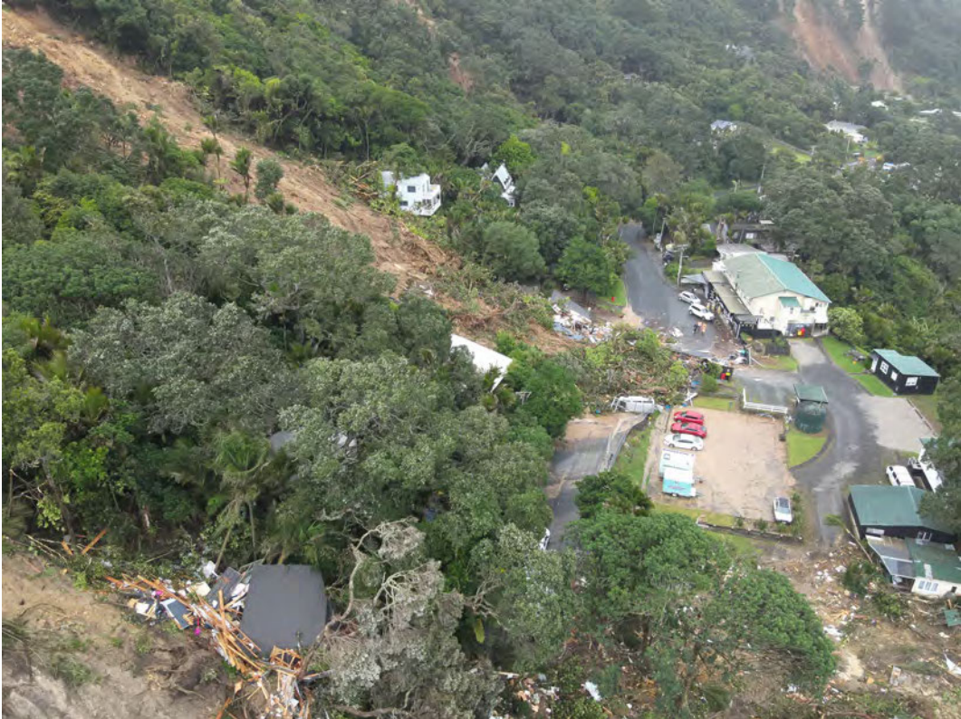
Figure 3 above. Rescue site in centre right where debris crosses the road. The landslide in foreground happened during the rescue approx. 1 hr 50 mins after the first landslide occurred. (USAR photo taken 14:00 hrs on 14 Feb)
