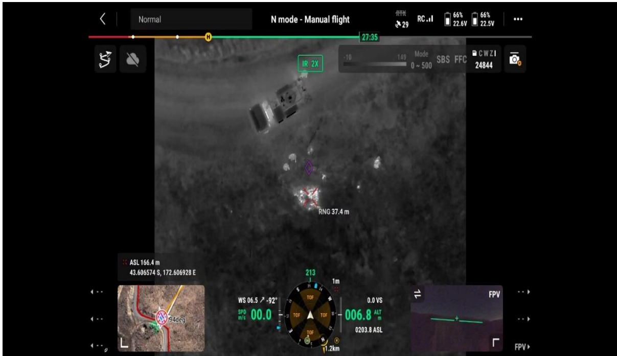
Fig 9 - Use of thermal camera to walk ground crews into difficult to find hot spots for extinguishment
