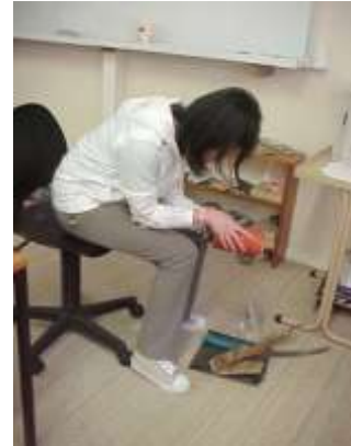
Sanding a sample to count the rings
