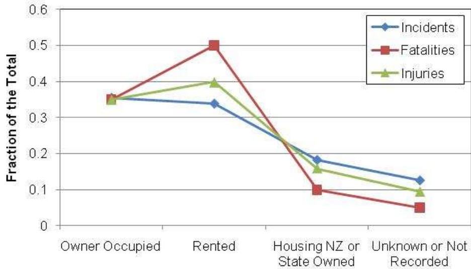
Figure 9: Fraction of the total fire incidents, civilian fatalities and moderate to severe injuries that occurred in unattended cooking fire incidents originating in the kitchen area for variation types of residential occupier. Adapted from New Zealand Station Management System incident data, 2002 – 2008, (Challands 2009).
