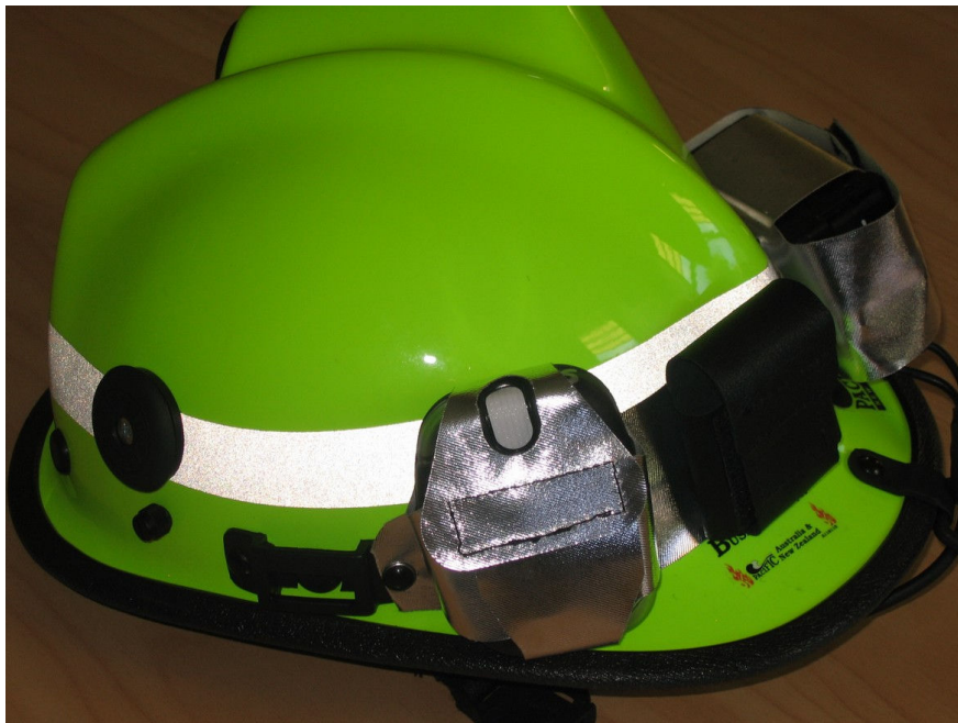
Figure 1 - Data collection helmet worn by firefighters. From the left are the CO monitor, GPS monitor and video recorder. Video camera is mounted on the right side of the helmet in the enclosure designed for a flash light.
