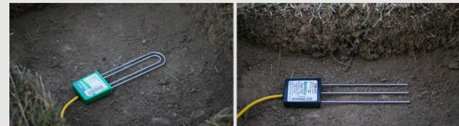
Sensors pictured above measure soil moisture and temperature every 10-30 minutes
