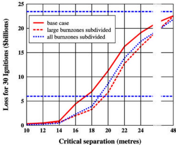
Figure 18: Effect of creating additional firebreaks on 50<sup>th</sup> percentile losses arising from 30 ignitions. The dashed line is the loss when large burn-zones are each divided into 3 equal portions, and the dotted line is the loss when all burn-zones are divided into 2 portions.
