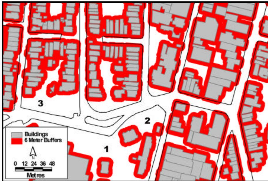
**Figure 9:** Examples of burn-zones for a mixed residential/commercial area of Wellington as defined by a critical separation of 12m. Fire is allowed to spread from one building to another when the separation is 12m or less, i.e. whenever there is contact between the 6m-wide buffer zones around adjacent buildings.
