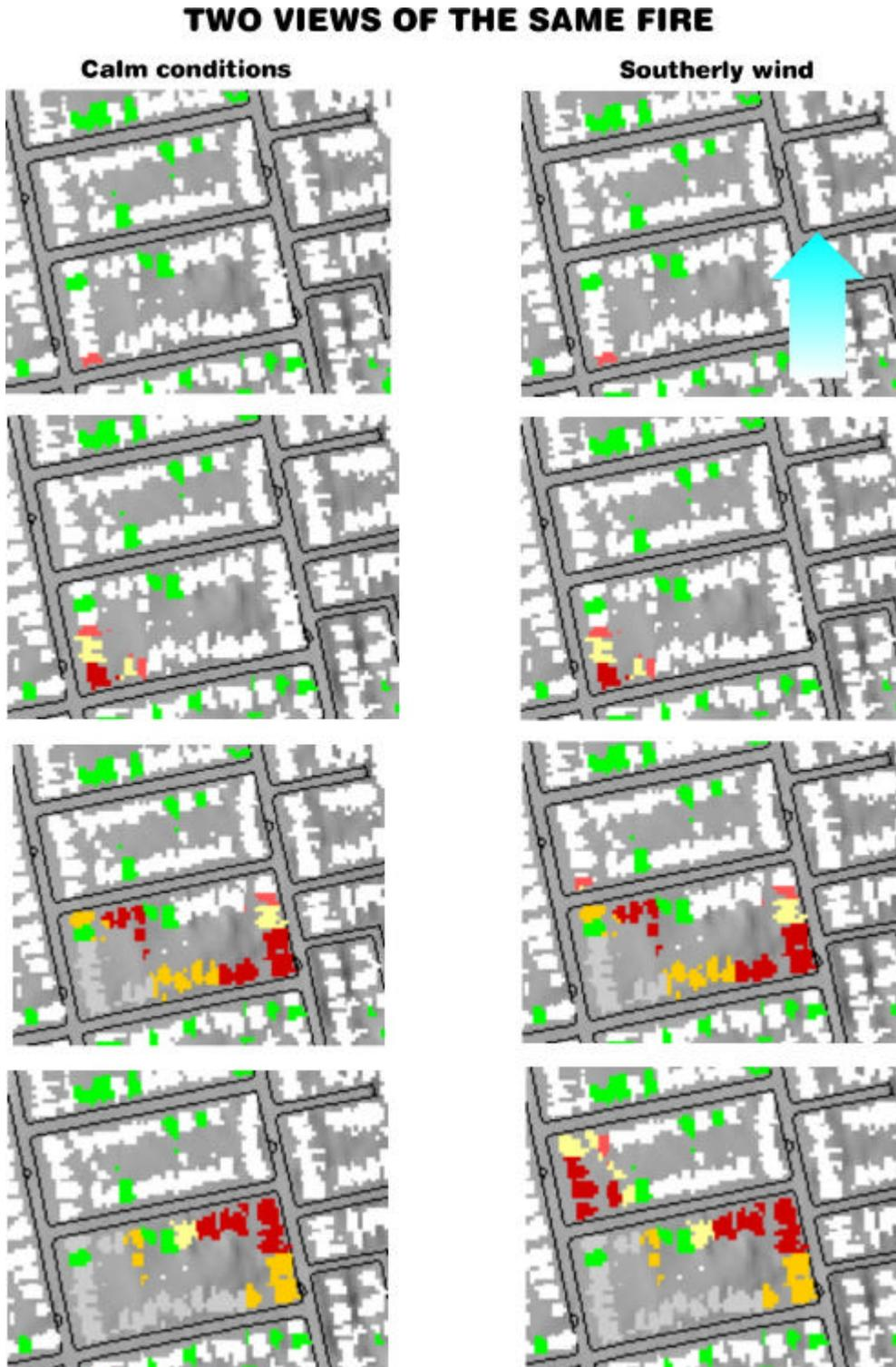
**Figure 8:** Example of visual display from the dynamic fire-spread model. The left-hand sequence shows the spread of a fire in calm wind conditions. The right-hand sequence shows a southerly wind causing the fire to spread across a road (third image from top).
