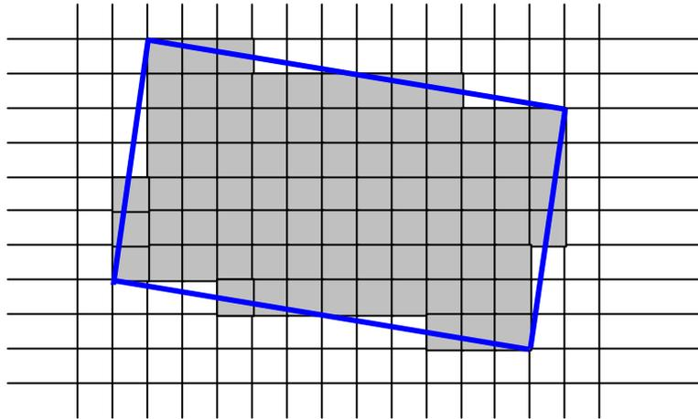
**Figure 3:** Allocation of properties to cells in the fire-spread model. The shaded cells are the ones allocated properties appropriate to the building denoted by the heavy outline.
