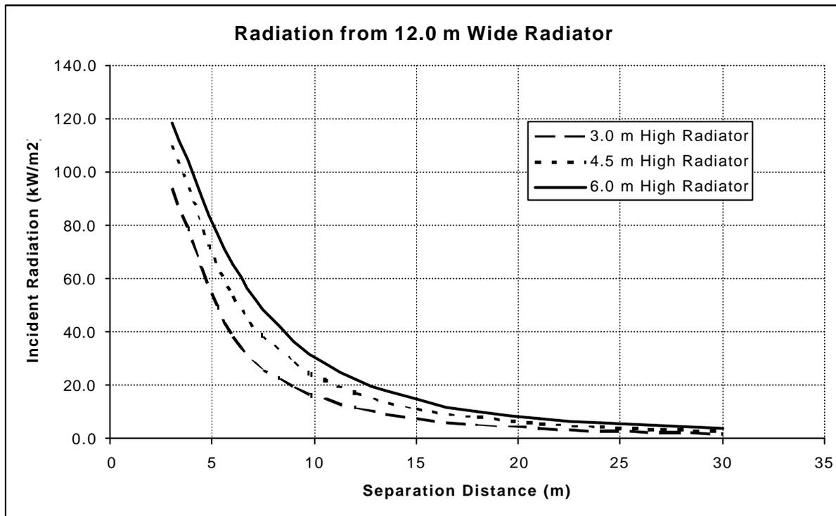
Figure 6. Radiation levels from radiators of various heights
