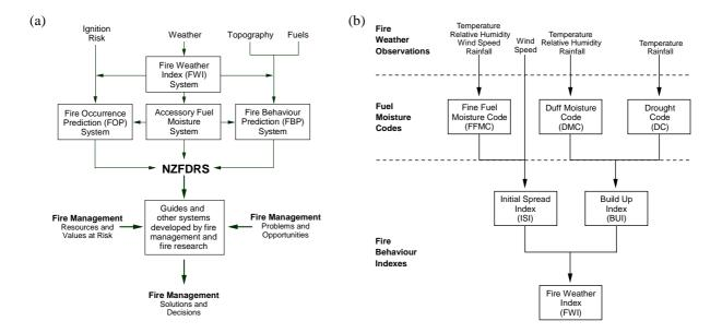
**Figure 2.** Simplified structure diagrams for (**a**) the New Zealand Fire Danger Rating System (NZFDRS), illustrating the linkage to fire management actions (after Fogarty *et al.* 1998); and (**b**) the Fire Weather Index (FWI) System (after Anon. 1993).
