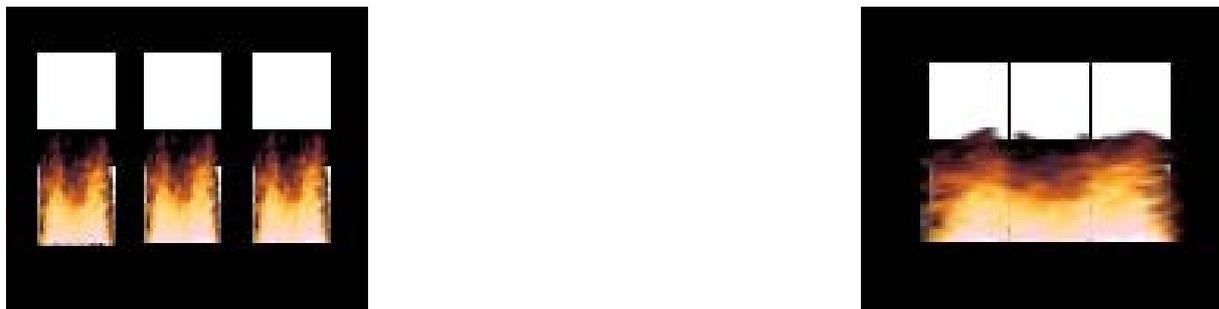
Figure 2.6 Typical layout of windows (left) and layout assumed for calculating the configuration factor (right).
