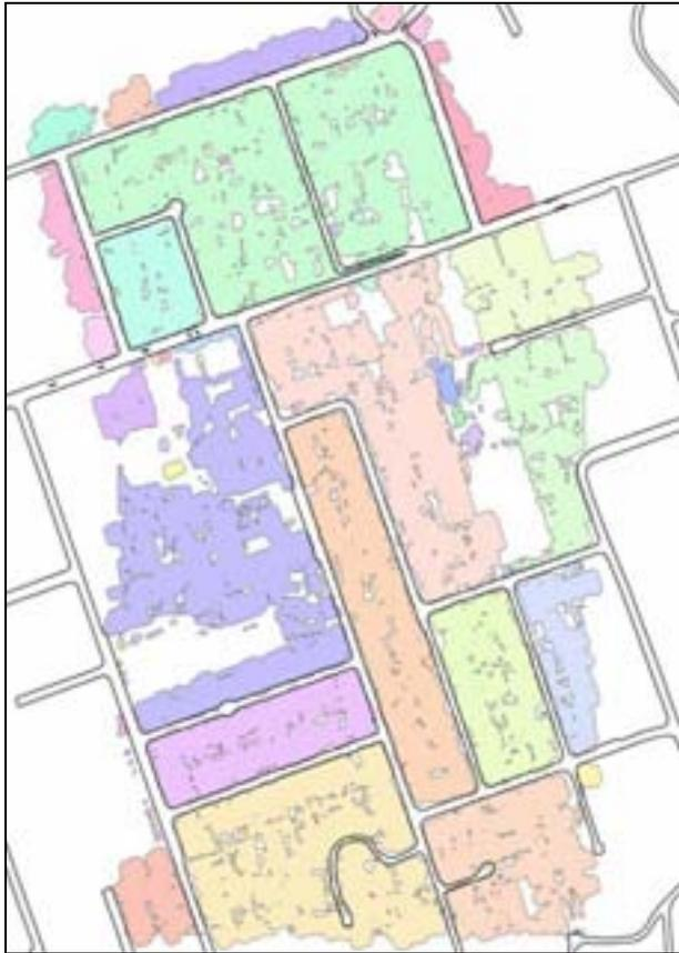
**Figure 3.6a** Burn-zones developed for critical separation of 10m on buildings and 2m on vegetation.
