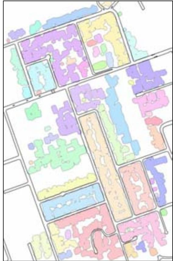
**Figure 3.6b** Burn-zones developed for critical separation of 10m on buildings alone.
