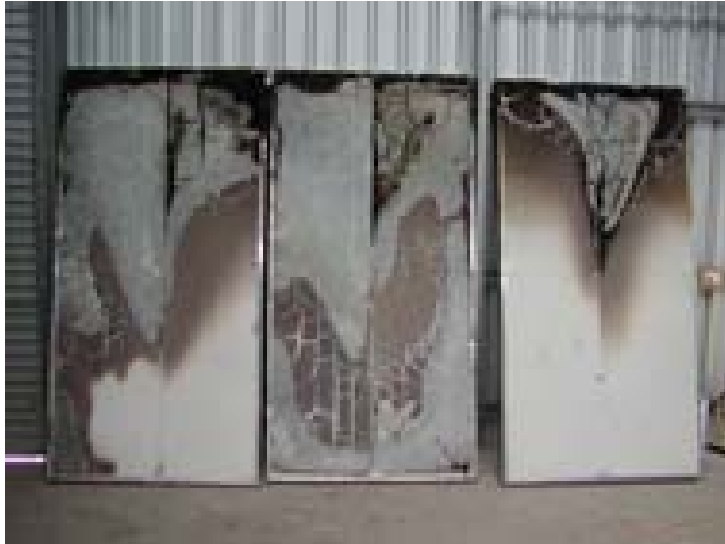
Figure 4.48: Interlocking joint specimens, unexposed side, trials 1 to 3 from left to right.
