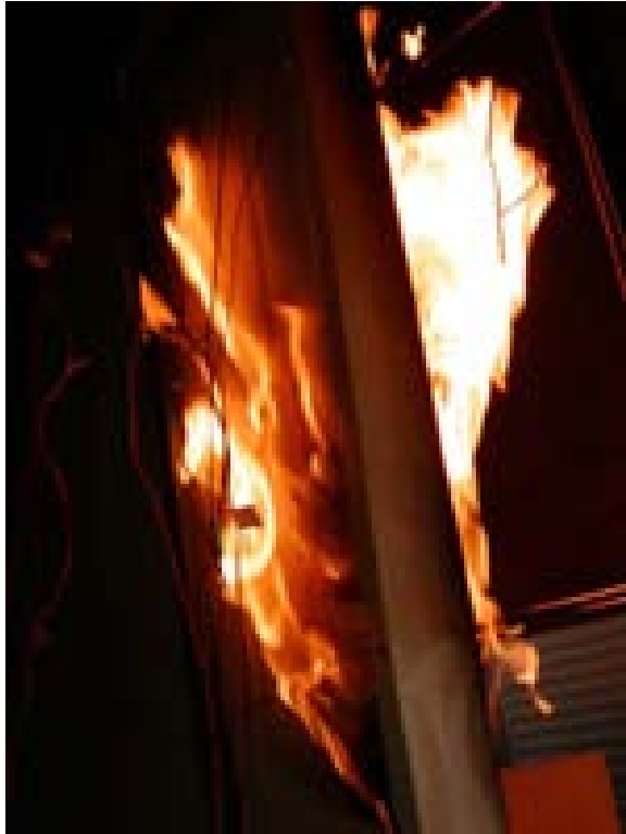
Figure 4.15: Trial 2 at 60 minutes exposure, flaming on the unexposed side (left in picture) due to ignition of gases escaping from gaps in edge capping.
