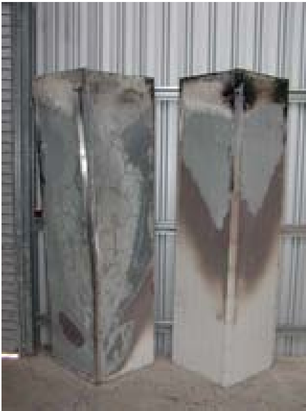
Figure 4.50: Corner joint specimens, unexposed side, trials 4 to 5 from left to right.
