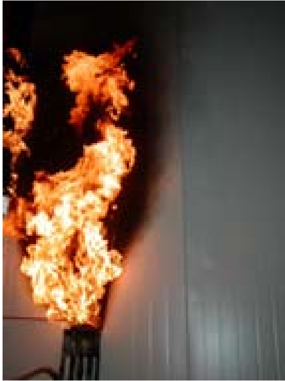
Figure 4.13: Trial 2 at 30 minutes exposure 300 kW (reverse angle) taken from RHS front side of specimen.
