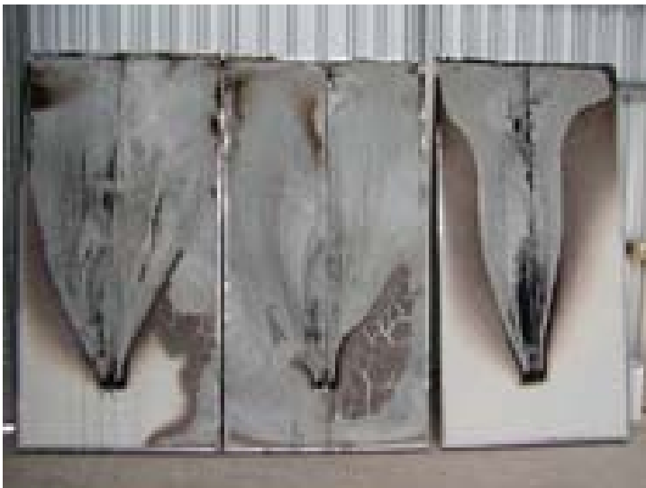
Figure 4.47: Interlocking joint specimens, fire exposed side, trials 1 to 3 from left to right.
