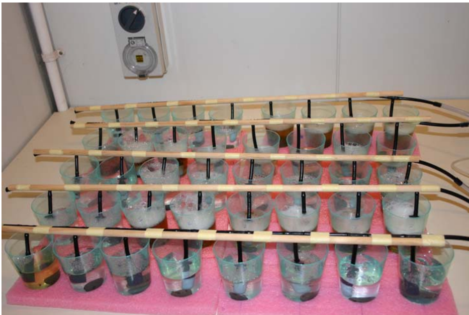
Figure 2. Experimental set up of the aquatic toxicity tests with mayfly larvae.
