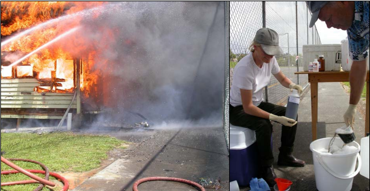
Figure 4: Fire-water collection from the St Mary's School tennis shed. Left: Fire-water flowing overland to tennis court stormwater drain (bottom right of photo). Right: Fire-water being bottled for contaminant analysis and toxicity testing.
