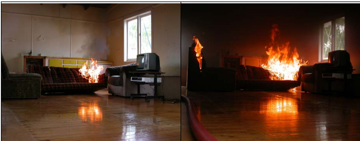
Figure 2: Mimicking a typical house fire using the St Mary's School tennis shed. Left: Fires were set to mimic a typical couch fire. Right: Mid-way through the first fire exercise, approximately one minute before this fire was extinguished.
