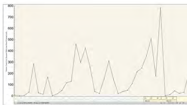
Figure 2: Graph of Hanmer predicted grass fire spread rate for the past month based on observed weather conditions.
